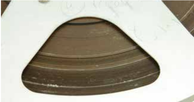
Damaged by bonding phenomena and in some cases affected by mold too
