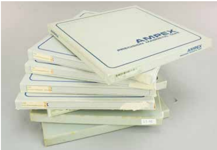
Magnetic tapes with different equalizations, speeds, tracks (CCIR / NAB - 7.5 ips / 15 ips - 2 / 4 tracks)
